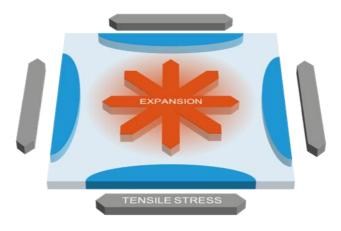
Figure 1 - Illustration of Thermal Stress Generation
