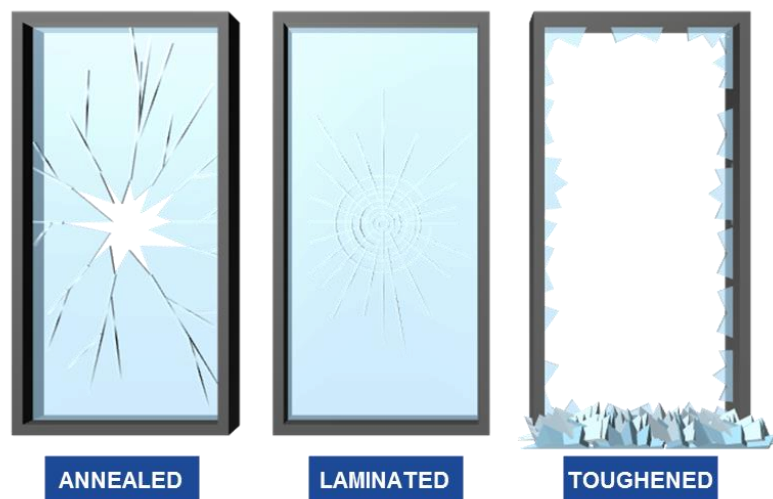
Figure 1 - Illustration of glass modes of breakage
