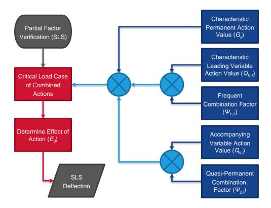
The effects of the actions, as well as being dependant on the combination of actions, will also be dependent upon the glazing construction on which the actions are taking place. As such, the determination of the ULS Stress and SLS Deflection will be dependent on the glass types and thicknesses, which will also influence the resistance to the actions.
