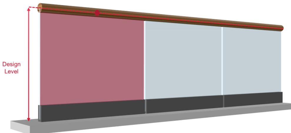
Figure 1 – Load application for a free-standing barrier with a handrail
