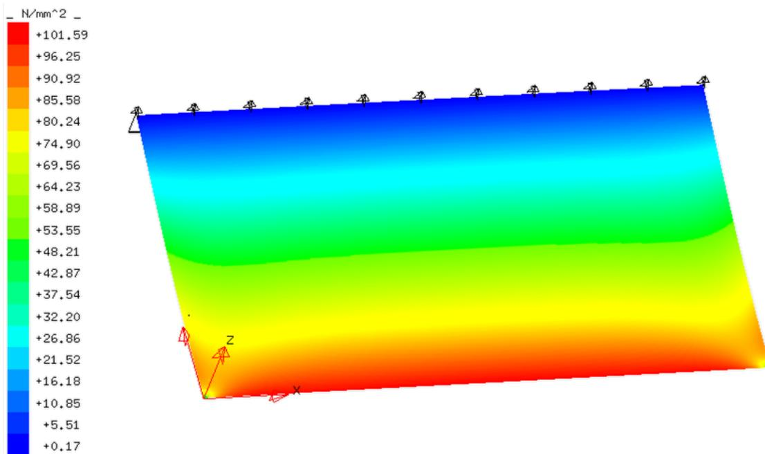
Figure 3 - Stress concentration for a bottom edge clamped free-standing barrier
