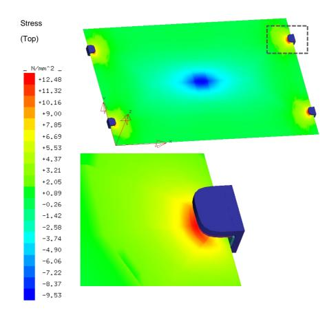
Figure 5 - Stress concentrations in glass around clamp finxings
