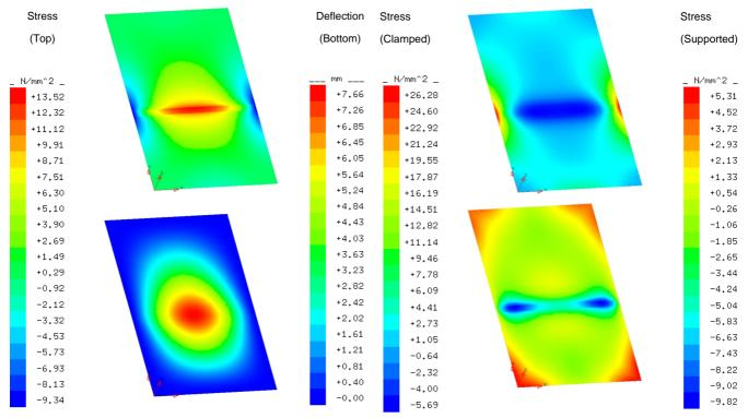
Figure 2 – Load distribution with clamped edge supported glass
