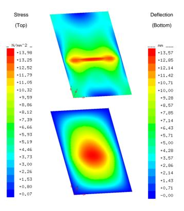
Figure 1 – Load distribution with simply supported glass
