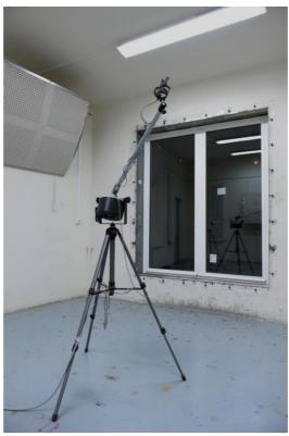
Figure 1 - Test setup for acoustic measurement
