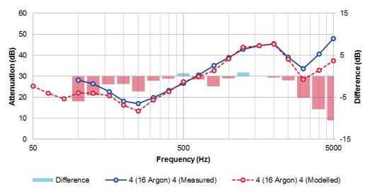
Figure 1 - 1/3 octave centre band performance data, modelled and measured, 4(16)4
